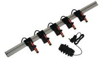
Designed for multi-blade rip saws or grading stations, this track/stationary bracket kit can accommodate any number of lasers. The lateral position of the lasers can be adjusted with a simple turn of a thumb screw. Each power supply distribution unit is able to accommodate up to 8 lasers, making service easy and requiring only one plug-in.
