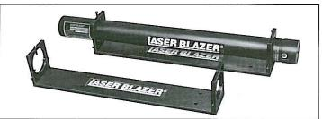
This optional mounting bracket is fastened to any stable surface with screws or bolts. It holds the LASER BLAZER linemaker firmly in position. Screw adjustments permit fast and easy movement of the linemaker laterally, or rotation to aim the laser line for maximum visibility and sharpness over the entire length of the boards to be sawed.
